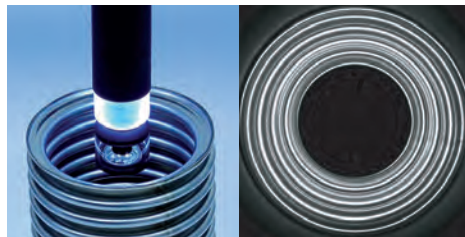
Tube scanning for integrity inspection
