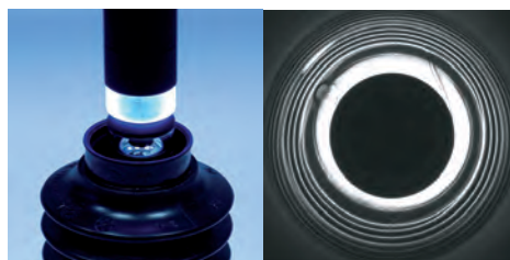
Rubber sealings control for leak prevention
